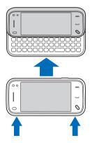
Your device has a full keyboard. To open the keyboard, push the touch screen up. In all applications, the screen rotates automatically from portrait to landscape when you open the keyboard.
